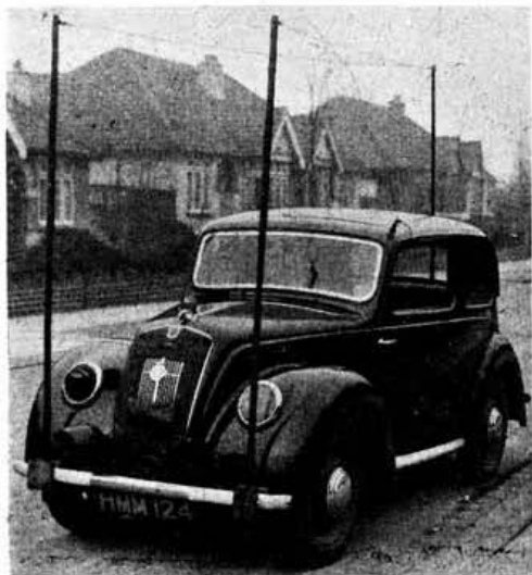
Portable operation was a feature of summer-time activities prior to the war. Here is the aerial system used by G8TL for some special tests which took place in East and South London on 1.7 Mc/s.
